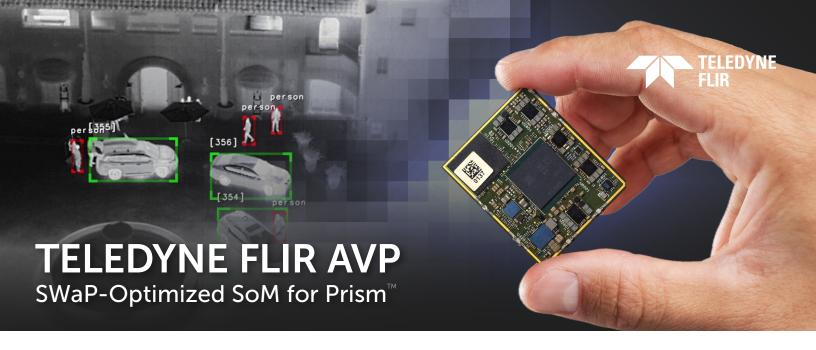
The AVP, a size, weight, and power (SWaP) optimized advanced video processor, provides best-in-class artificial intelligence performance for thermal infrared and visible camera perception systems. It incorporates the latest Qualcomm® QCS8550, the industry's most advanced mobile processor system on chip (SoC) featuring up to 48 TOPS inference compute performance. The QCS8550 is part of Qualcomm's Product Longevity Program, ensuring future-proof product stability.
