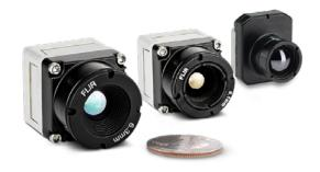
Made in the USA and ITAR free, the Boson+ sets the standard for longwave infrared (LWIR) OEM thermal camera performance and size, weight, and power (SWaP). It features an industry-leading thermal sensitivity of less than or equal to (≤)20 mK. The upgraded automatic gain control (AGC) filter and new DDE+ deliver dramatically enhanced scene contrast and sharpness. Lower video latency enhances tracking, seeker performance, and decision support.
